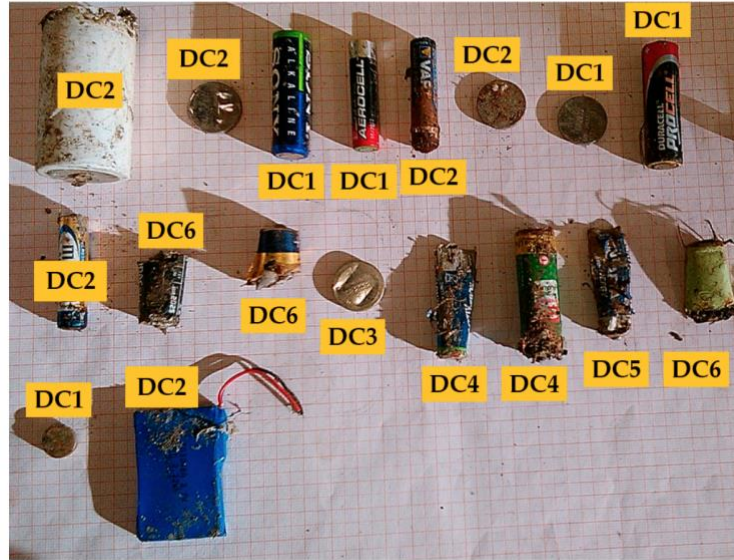
Figure S1. Damage classes of end-of-life portable batteries (after sampling campaign).
